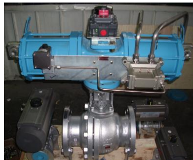
HIGH SPEED (1S) BALL VALVE 6" 300LBS FLANGED END FLOATING TYPE METAL SEAT
