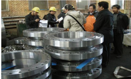
ASTM A694 F70 FLANGE 28" 600LBS WN RF SCH.14.28MM ASME B16.47 SERIE A
