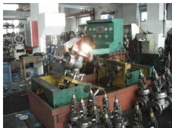
GATE VALVE LEAK TEST
