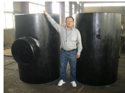
ASTM A860 WPHY 65 BUTT WELD FITTING REDUCING TEE 32" x 26" SCH.0.75" x 0.688"
