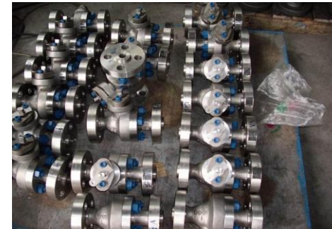
CASTED A351 CF8M 1" x ANSI 1500LBS FOR FABRICATOR SHELL IN MALAYSIA
